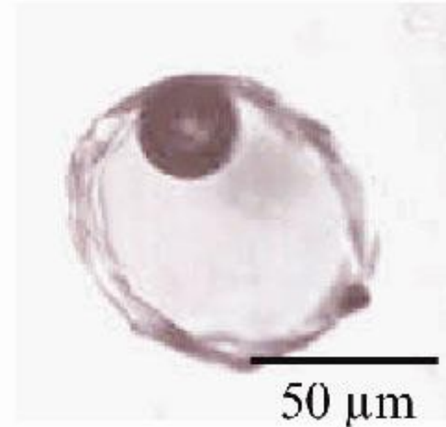
Microphotograph of one olivine-hosted glass inclusion (Stromboli sample). The silicate melt is trapped at high temperature during the olivine crystal growth and preserved as a glass inclusion within the mineral, upon cooling
